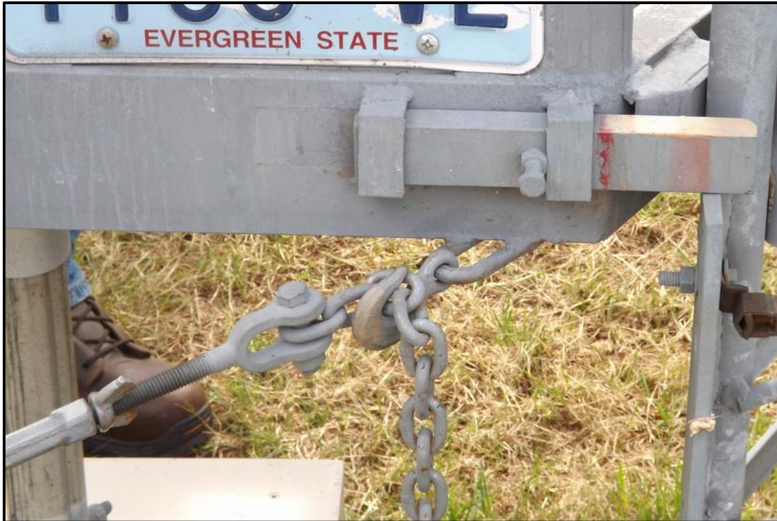
Figure 12 – chain affixed to pelican hook at rear of trailer frame – it will probably be fastened by a link close to the middle of the chain
