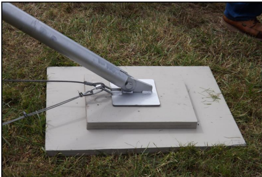
Figure 8 - Correct position of right outrigger pad when facing rear of trailer
