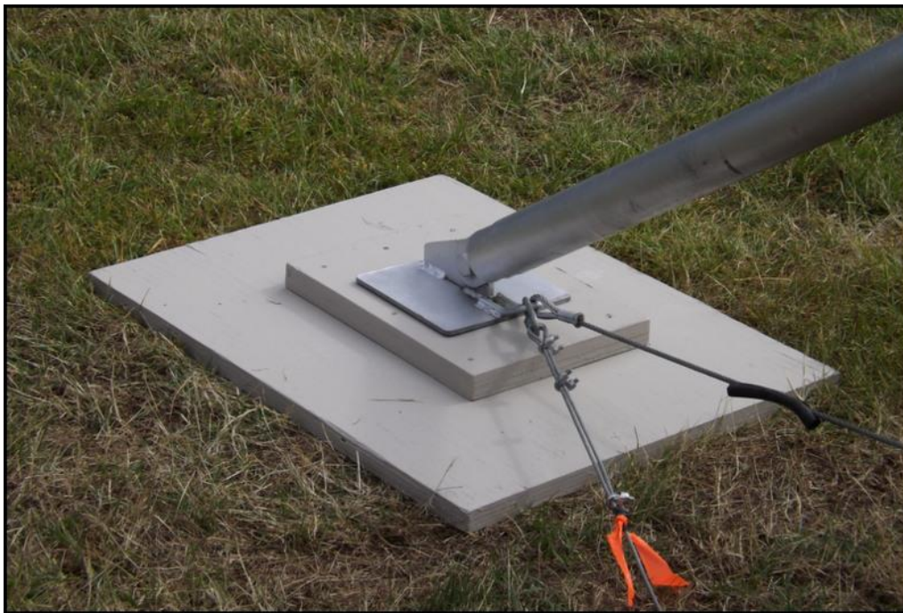
Figure 7 - Correct position of left outrigger pad when facing rear of trailer. Note the orange ribbon on the hobble cable
