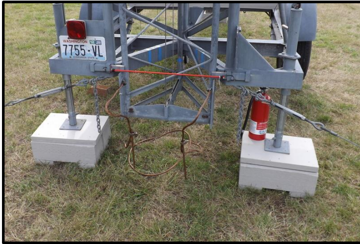
Figure 22 - Copper Ground Rods in Position
